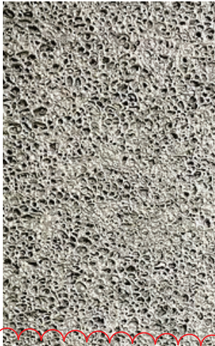
CL:01 Aluminium Stabilised Foam (Closed cell)
