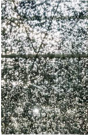
CL:02 Aluminium Stabilised Foam (Open cell)
